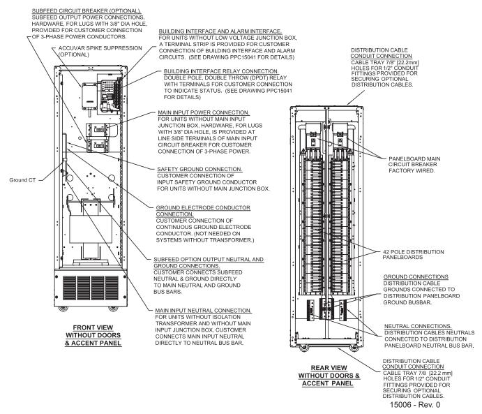
Figure 6 Electrical connection location for 47" (1194mm) cabinet—Front view
